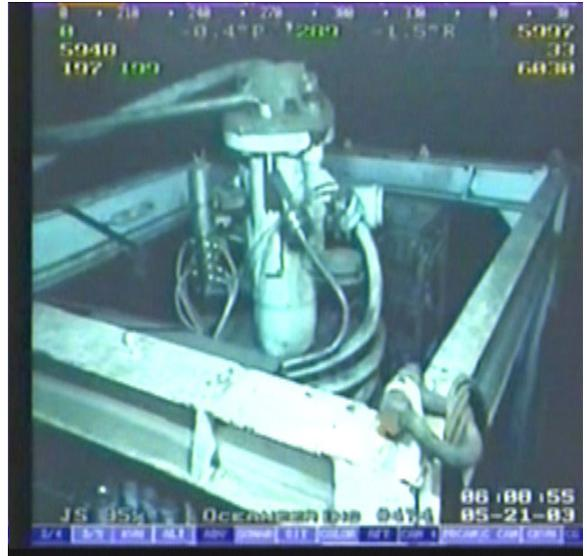
Figure 6. Photograph of lower marine riser package after the release. Note the lack of accumulated drilling fluid solids (frame from ROV video, May 21, 2003).
