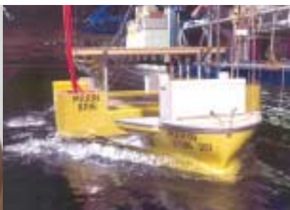
Modeltests of the Blue Marlin at MARIN.
