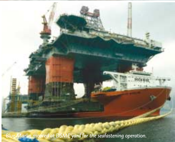
Thunder Horse positioned on deck of the Blue Marlin.
